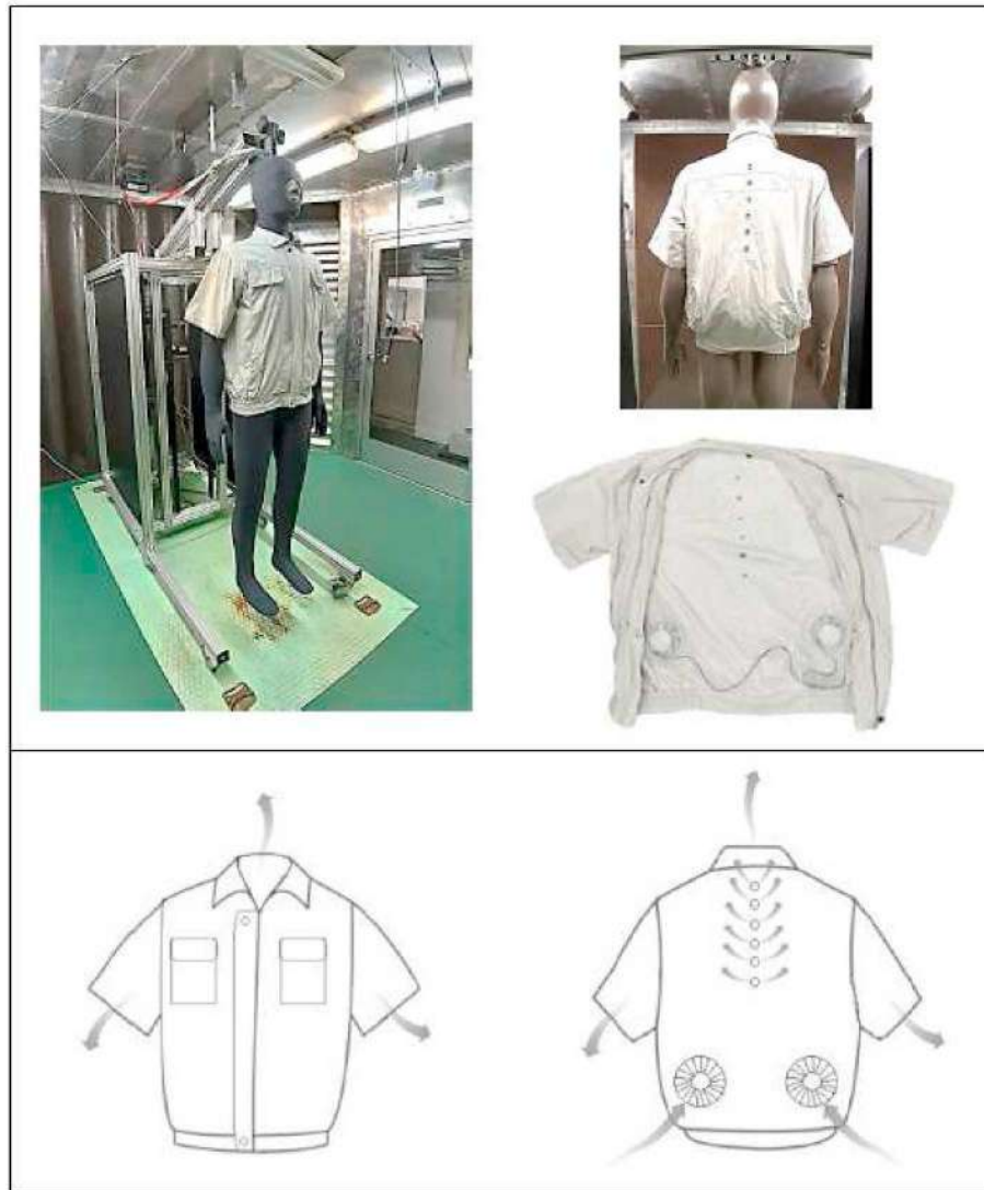
Fig. 1. The ventilation jacket tested with six circular openings and two fans placed in the back site.
